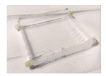
39. Carefully slide the gel off the gel tray directly onto the UV transilluminator for viewing and imaging.
