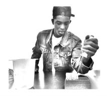
7. Use a small plastic micropestle to macerate your insect sample. Twist down and rotate with force to **crush it as much as possible**.
