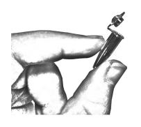
Add all reagents to the **side** of the PCR tube so you can see the droplet.
